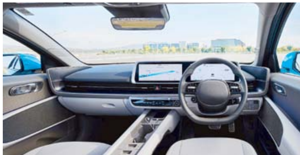
Despite being entry-level the Dynamiq is well equipped, with standard features including, head-up windscreen display, dual 12.3-inch display monitors, 10-way powered driver and front passenger seats, eight-speaker Bose audio, wired Apple CarPlay and Android Auto, multi-Bluetooth connectivity, Blue Link Connected Car Services and a powered boot lid.
